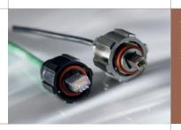
TE offers a broad range of USB connectors. The IP20 series features an integrated locking mechanism with audible and tactile feedback, creating an excellent interconnect solution for internal USB cable routing without having to worry about the plug coming loose during transit and use. A sealed and highly reliable version (IP65/IP67) for rugged and harsh environments is also available.
