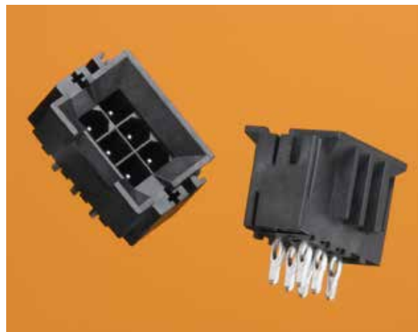
Mini-Fit® Compliant Pin Interface (CPI) vertical headers utilize a highly reliable "eye-of-the-needle" contact design, handle up to 8.0A current and are ideal in blind-mate and press-fit networking applications.
