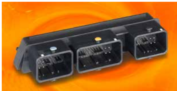
CMC 154-circuit header in compliant pin mount offers robust, sealed, wire-to-board connection for high-conductivity, high vibration powertrain applications.
