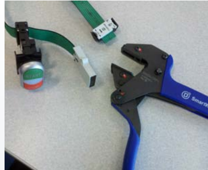
Eaton SmartWire-DT crimper, right, pushes the module closed over the flat wire. A connected Eaton pilot/pushbutton is shown, left. Courtesy: CFE Media
