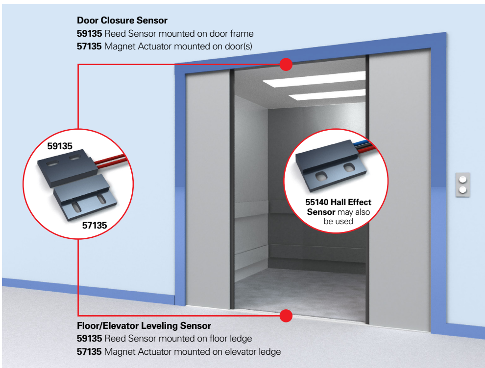
Figure 2. Reed Sensor Used in an Elevator Door
