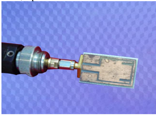
Fig12. The final fabricated dual band microstrip patch antenna
