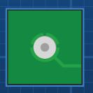
Thermals are small traces used to connect a pad to a plane for heat relief.
