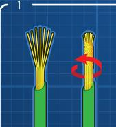
Strip 3mm of insulation from the stranded wire.
