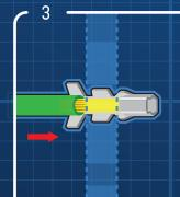
Place wire in up to the insulation, and crimp inner wings around the wire strands.
