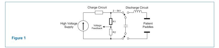
In this circuit R1 is a high value resistor, normally in the range 5M to 50M, which, together with a commodity chip resistor R2, forms a potential divider for voltage feedback.
