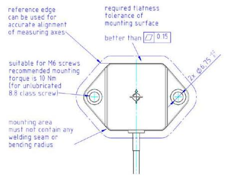
Figure 7. Mounting Detail
