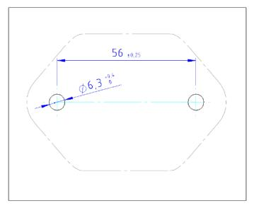
Figure 9. Mounting Hole Detail
