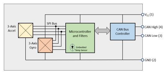
Figure 1. Block Diagram
