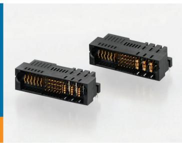
TE Connectivity's MULTI-BEAM XLE connectors are the latest addition to the MULTI-BEAM XL power connector product family. MULTI-BEAM XLE connectors feature a new 3-beam contact, made from a thicker (higher) conductivity material than the original single-beam or 4-beam designs. The new 3-beam design allows for a greater angular mis-alignment between mating connectors and offers a lower mating force.
