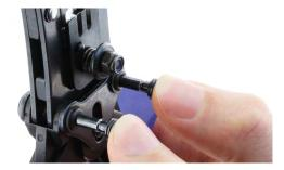
5) Place conductors, with no deterioration, in the contact bucket. All strands to be located in the crimp bucket.
