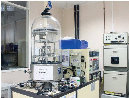
Vacuum bell for robotic operating testing -170°C/+200°C temperature gradient
