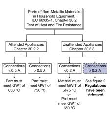
Figure 1: Overview of plastic components in electrical household appliances
