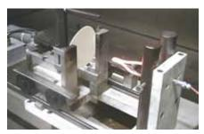
Figure 3: Glow wire test setup
