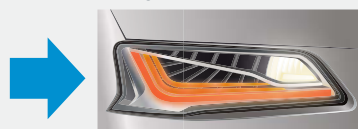
Design Combining LEDs with a Light Guide(Uniform Light Source) (No. of LEDs: Few)
