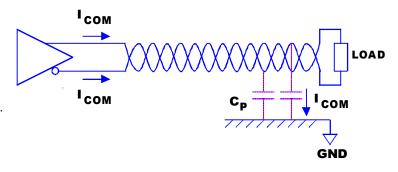
Common mode signals directly generate RFI in UTP cable systems.
