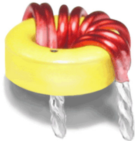
Fig. 1a. Wound toroid inductors were mainstay of desktop voltage regulators.
