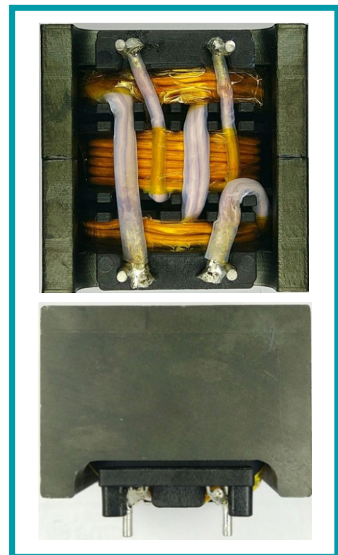
Fig. 9: Transformer prototype sample.
