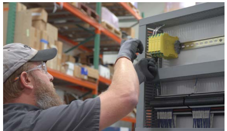
Figure 3: Safety relays with force-guided contacts are SIL-certified.
