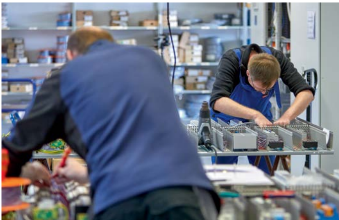
Figure 2: System integration experts create complex control cabinets.
