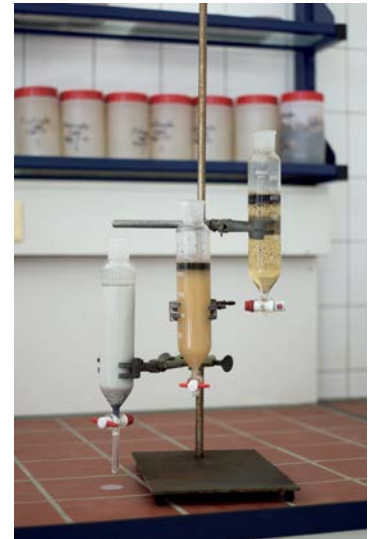
Figure 3: Illustration of the emulsion separation process in the lab.
