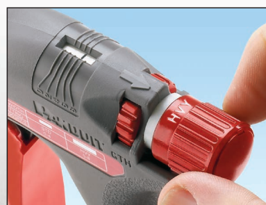
Recommended tool setting of HVY 4-6 – Less force required to properly secure the cable tie.
