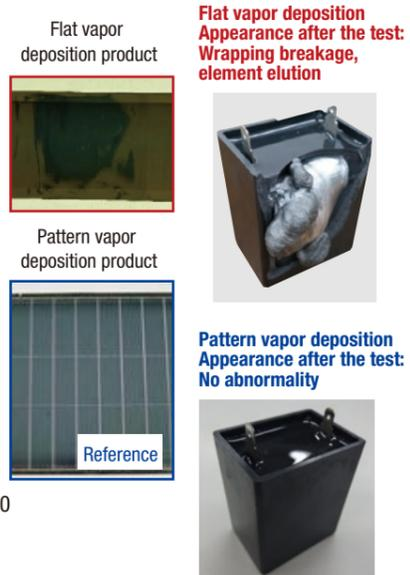
\* In this test, the test power supply is shut off by detecting the short mode with the overcurrent, but there is a possibility of burning or fire if it is not shut off.
