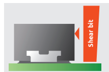
Figure 9: Board level robustness improvements of DFN packages with side-wettable flanks
