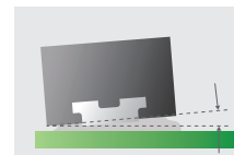
Figure 9: Board level robustness improvements of DFN packages with side-wettable flanks
