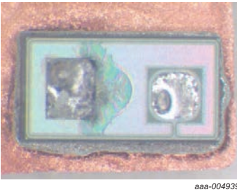
Fig 57. Sample image 66; 20 V, 3 A, 60 ms
