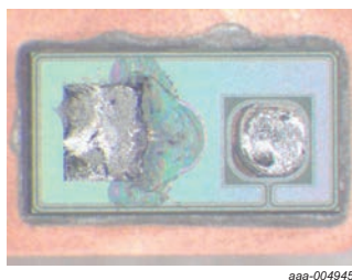
Fig 63. Sample image 73; 30 V, 1.4 A, 60 ms
