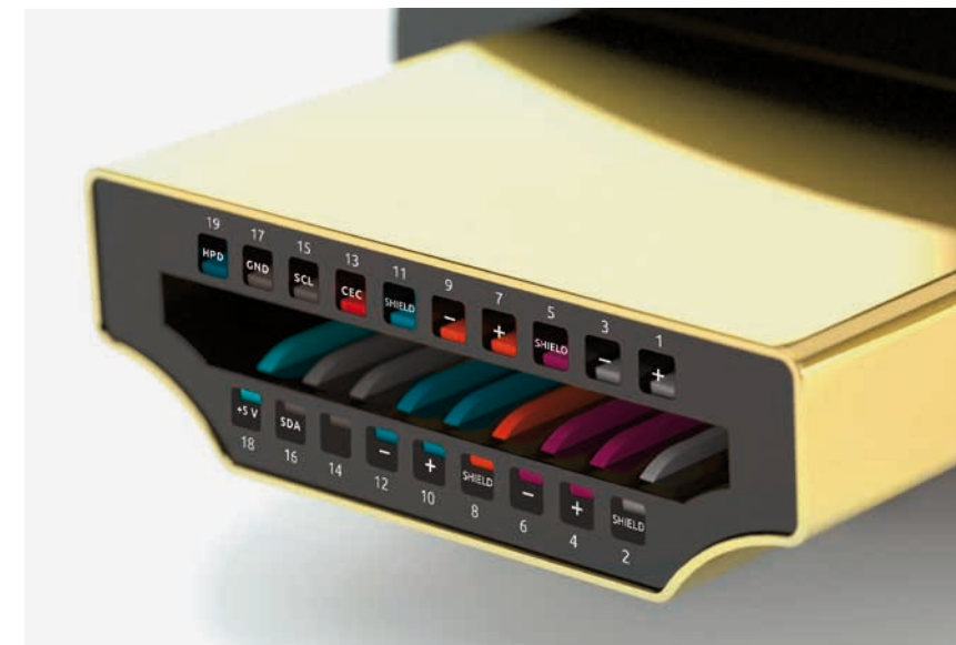
Figure 81 | Pinout and front view of HDMI connector
