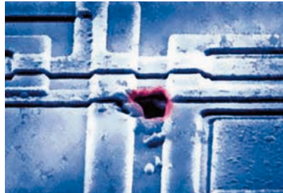
Figure 64 | Example of ESD damage
