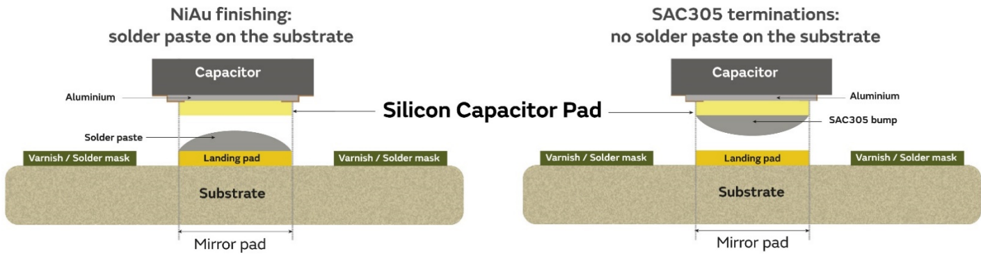
Figure 8: Simplified view of NSMD assembly from the side (only one pad is shown here)
