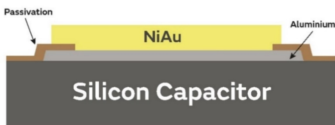
Figure 1: Left side - Simplified view of a Si-cap pad for reflow; right side – SEM view of a Si-cap with SAC305 terminations
