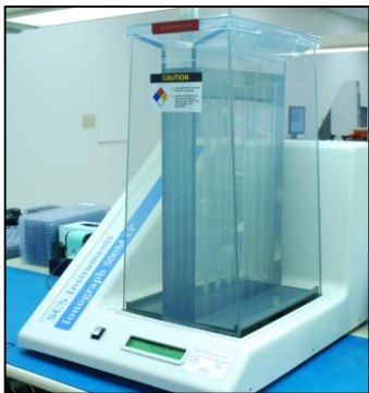
Ionograph Cleanliness Testing
