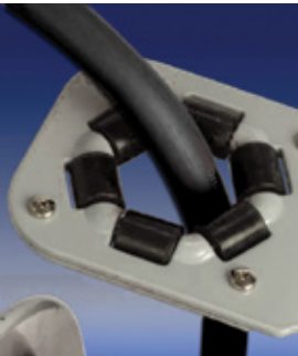
Six-roller design minimizes hose wear.
