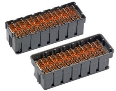
NeoPress ® High-Speed Mezzanine SystemTop: Plug, Bottom: Receptacle6-by-14 (84 triads)
