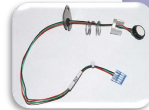
Value Add 1865 Series Force Sensor assembly with custom packaging
