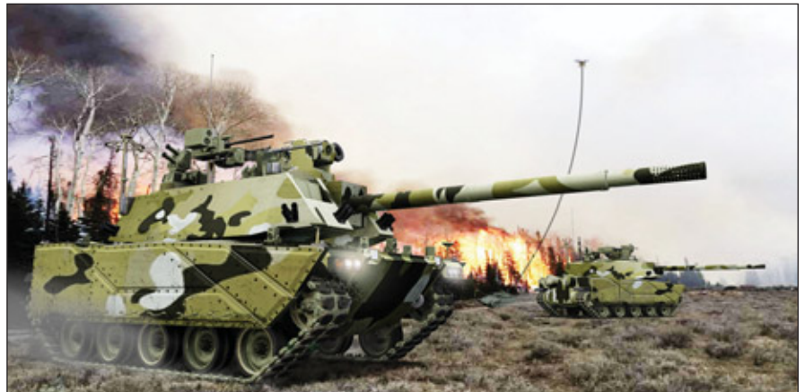
The Next Generation Combat Vehicle's manned-unmanned teaming concept would leverage a protected tether between the NGCV Optionally Manned Fighting Vehicle and the Robotic Combat Vehicle in order to give soldiers the capability to safely engage in combat with autonomous systems while safely remaining outside of enemy range. (Photo Credit: U.S. Army)
