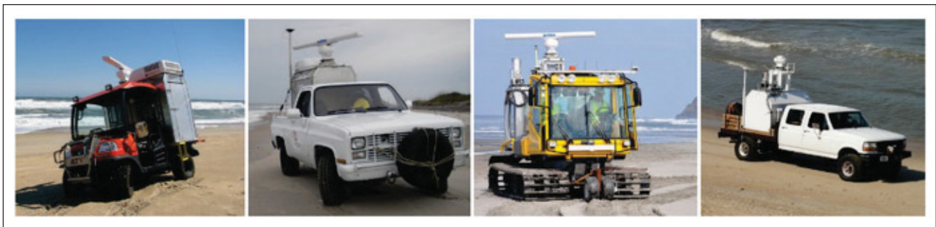
The progression of the Coastal LiDAR and Radar Imaging System (CLARIS) research and development through the years 2007- 2016, left to right: Kubota UTV, Chevrolet Blazer, Prinoth track vehicle, and Ford F350 truck.
