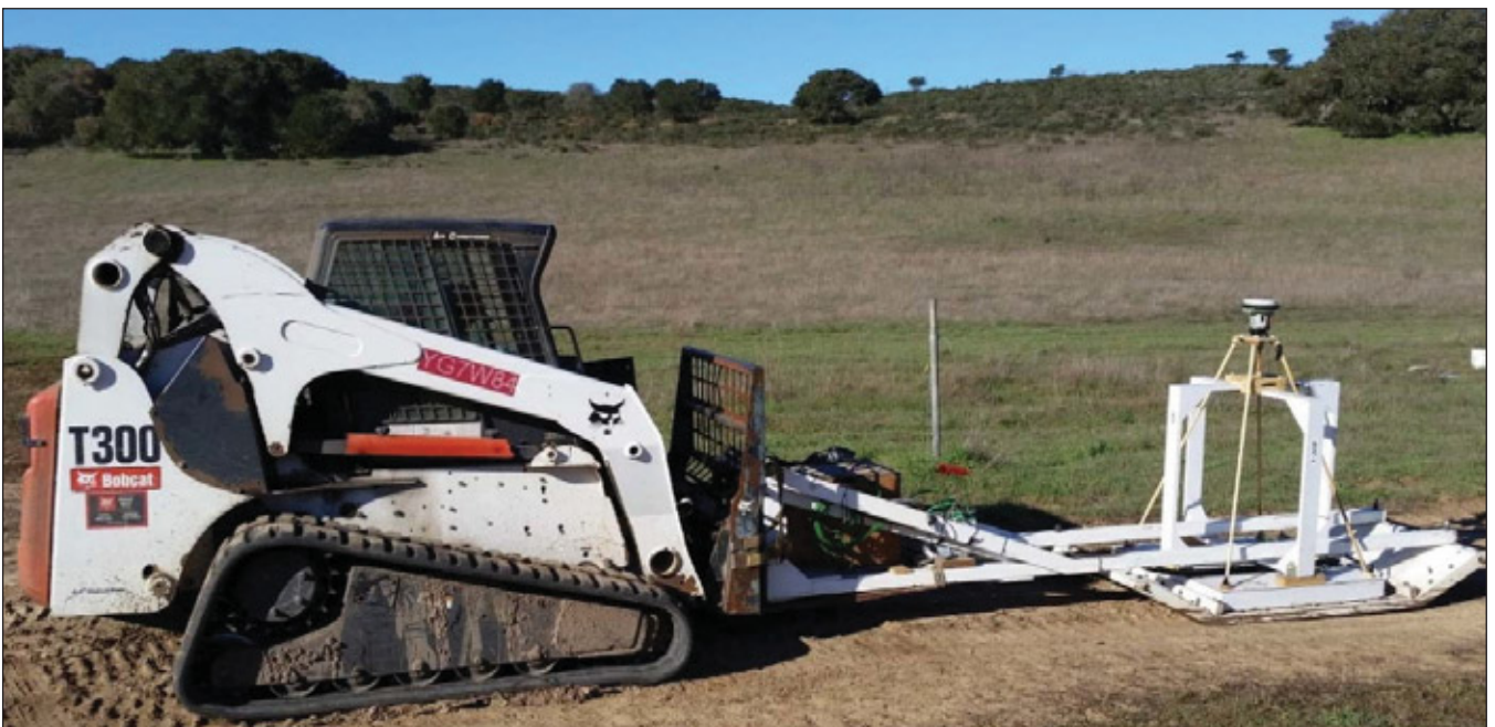
MetalMapper (MM) Configured for Cued Data Collection with Bobcat
