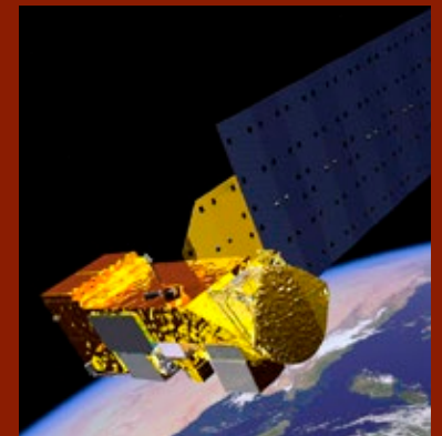
Satellite plating with gold is used when insulation alone is inadequate to protect the satellite from radiation from heat, light, and impact. Gold is effective in reflecting radiation away from the satellite, is a good heat and electrical conductor, and does not react to atomic oxygen.
