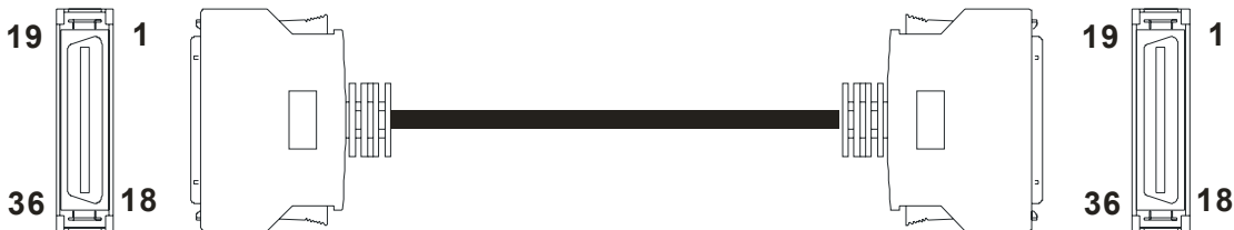
Figure 12 UC-ET010-13B ( 1M ) Female MDR36 connector ↔ Female MDR36 connector
