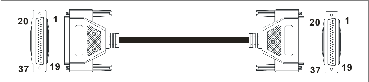
Figure 6 UC-ET010-33B (1 m) Male DB37 connector ↔ Male DB37 connector
