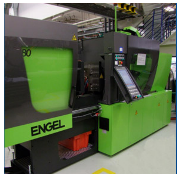
Production of Delphi Gum Based Silicone Rubber Sealing Components in Wuppertal, Germany facility, which uses a different process from liquid silicone rubber.
