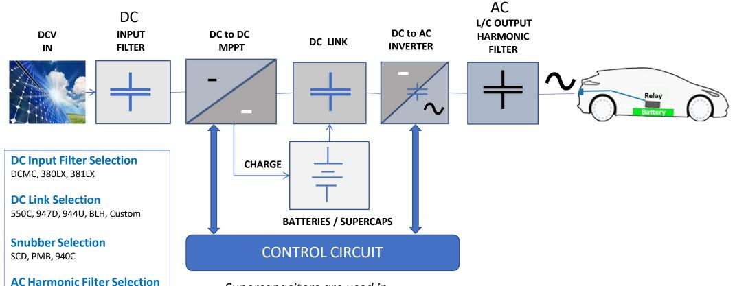
Supercapacitors are used in combination with batteries for energy storage from solar inverters.
