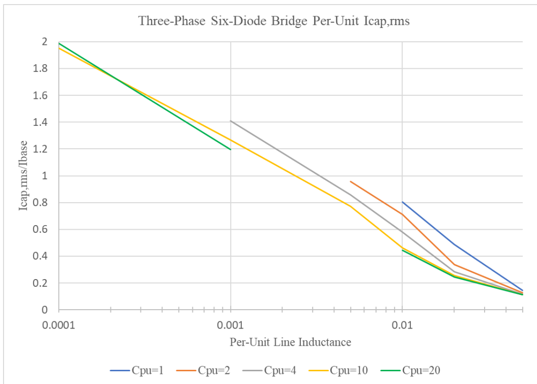
Figure 13: Per-unit analysis of RMS ripple current through the filter capacitor versus line inductance for five values of filter capacitance.
