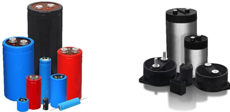
Figure 1 shows some of Cornell Dubilier's DC Link capacitors for power inverters. Left photo features aluminum electrolytic capacitors of snap-in, plug-in, and screw-terminal varieties. Right photo shows screw-terminal, stud-terminal, and solder-leaded film capacitors.
