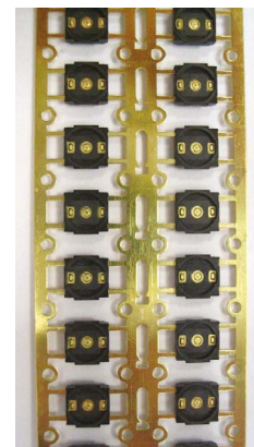
Precision stamping and over molding tools designed and built by C&K
