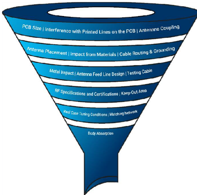
Figure 11: Antenna integration considerations for successful wireless design (Source: KYOCERA AVX)
