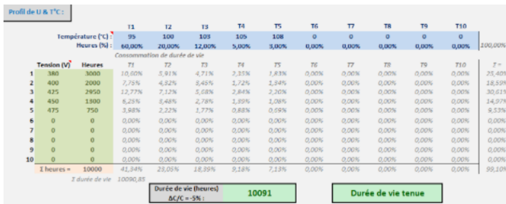
Figure 5. Hotspot simulations for various voltages to determine capacitor lifetime
