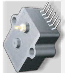
A 6 C B J A-Package Six (6) leads Two (2) ports cut 0.100" Barb fitting, port 'A' only Jogged lead bend
