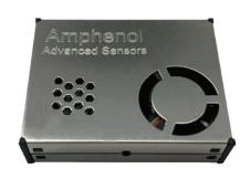
SM-UART-04L Particulate Dust Sensor is designed for a wide range of air quality applications where fine particle dust needs to be measured. Applications include air quality meters and air purifiers for both residential and light industrial monitoring and control. The optical design leverages laser technology, which allows customers to achieve excellent performance with balanced reliability. SM-UART-04L is an ideal solution for industrial and consumer applications.
