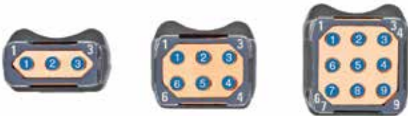
Using Socket (Female) Contacts
