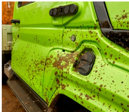
With protective caps inserted: IP6K6K/IP6K9K
