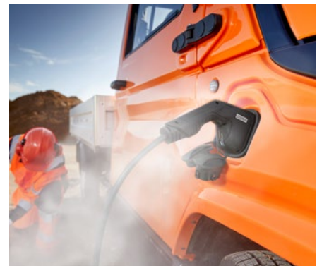
With charging connector plugged in: IP44B/IP44D
