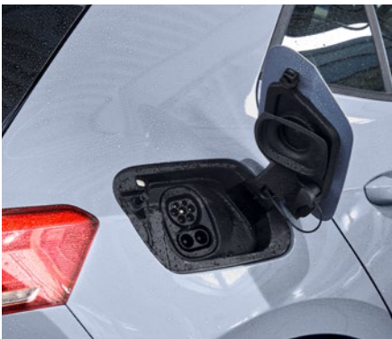
With vehicle charging inlet uncovered: IP6K6K/IP6K9K
