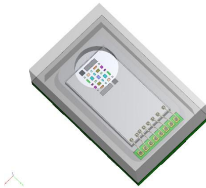
Figure 7: The TCS3448 spectral sensor!
