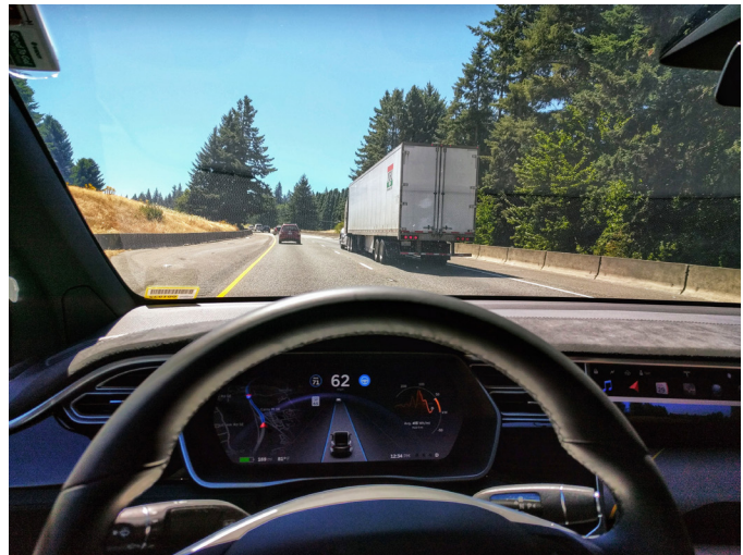
Figure 2: SAE Level 2 systems like the Tesla Autopilot, seen here controlling distance from the lead car and centering the vehicle in the lane, need large amounts of data to enable rapid decision-making.
