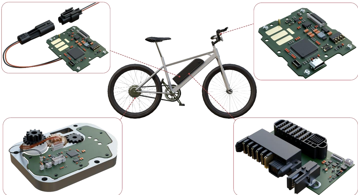
Squba connectors within an e-bike. (Image courtesy of Molex.)
