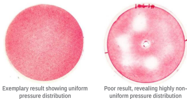
Figure 10: Results from inspecting the Pressure Distribution using Color-changing Film
