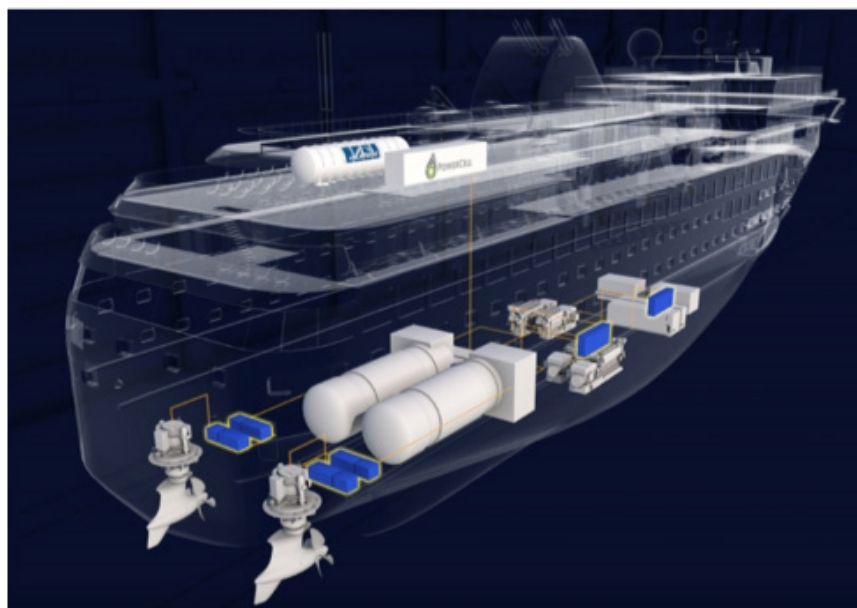
Figure 6. Cross Section of a Hydrogen Powered Ship
