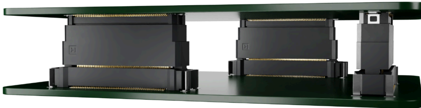
Figure 1: Applications with multiple board-to-board connectors are the most challenging from a connector placement perspective
