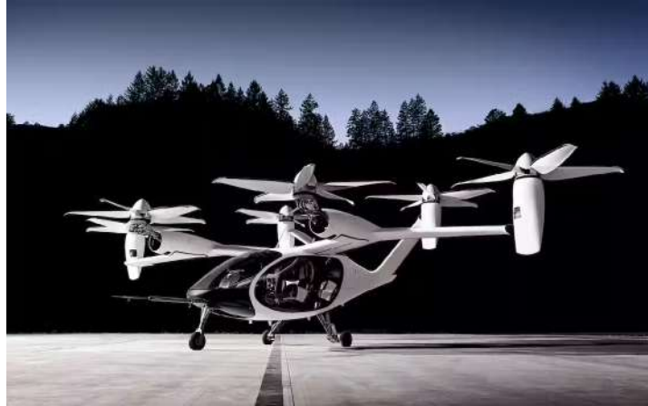
Figure 1: The Joby Aviation S-4 all-electric eVTOL, which has six electric motors to carry one pilot and four passengers, was awarded military airworthiness approval in 2020, and recently established a new certification agreement with the FAA for a more rapid commercial entry date of 2024. Image used courtesy of Joby Aviation
